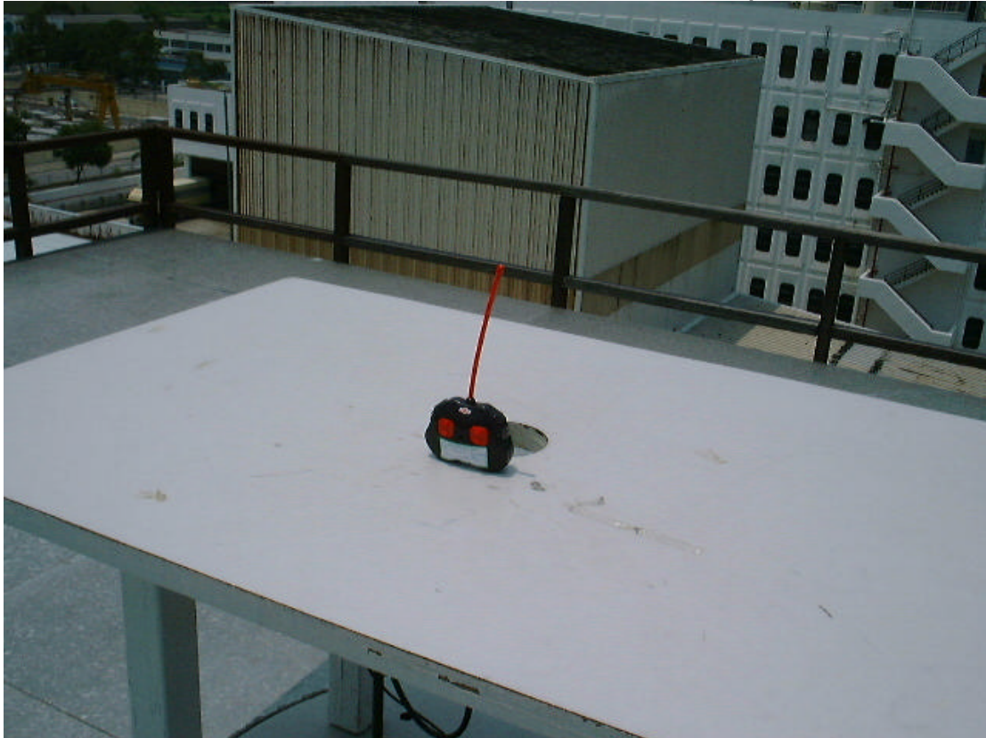
Measurement of Radiated Emission Test Set Up
