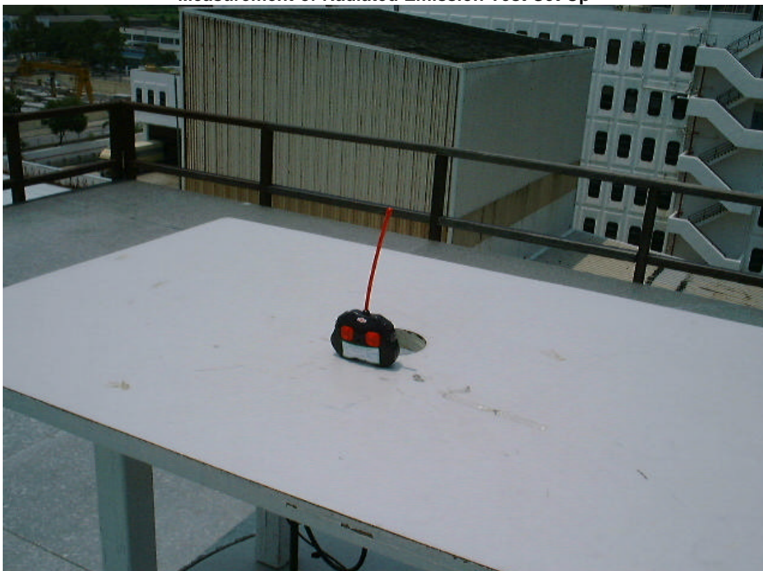
Measurement of Radiated Emission Test Set Up
