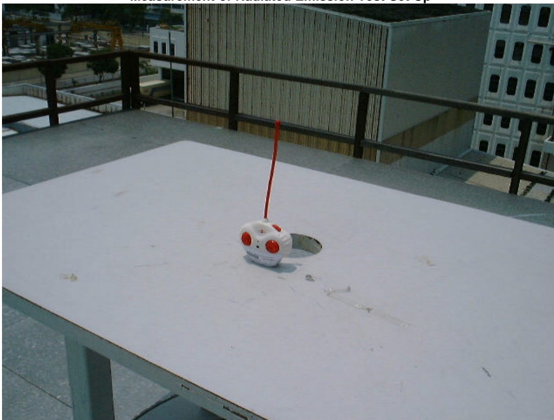
Measurement of Radiated Emission Test Set Up
