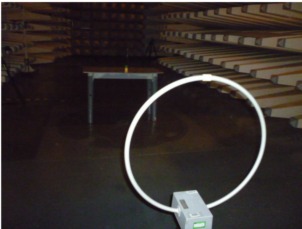
Set-up for Radiated Emission (Transmitter)
