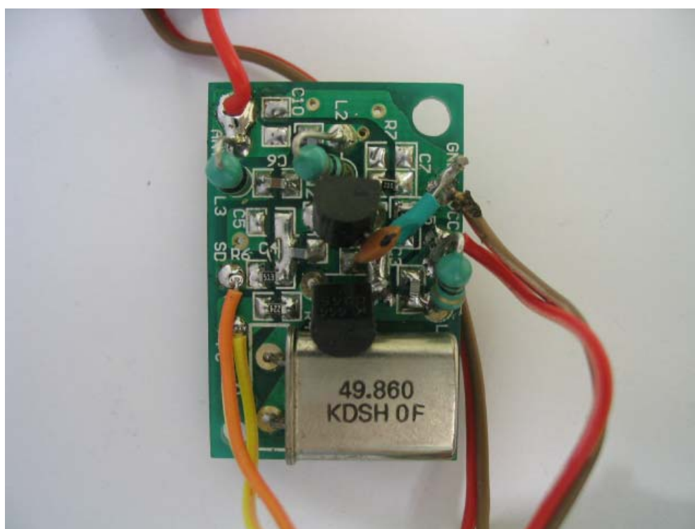
Transmitter (Internal view)
