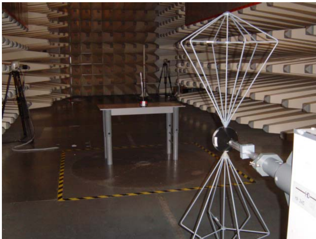
Test Setup for Radiation Emission
