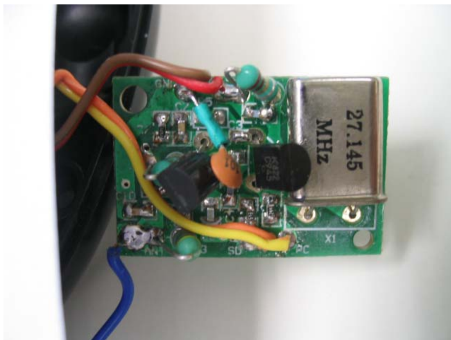
Transmitter (Internal view)
