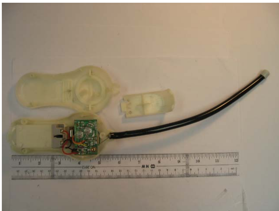
Transmitter (Internal view)
