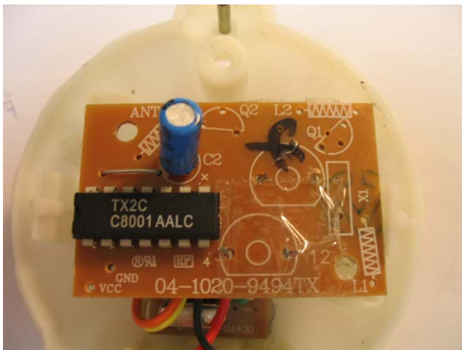
Transmitter (Internal view)
