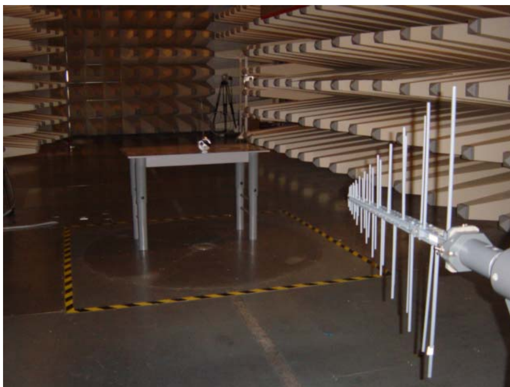
Set-up for Radiation Emission (Transmitter)
