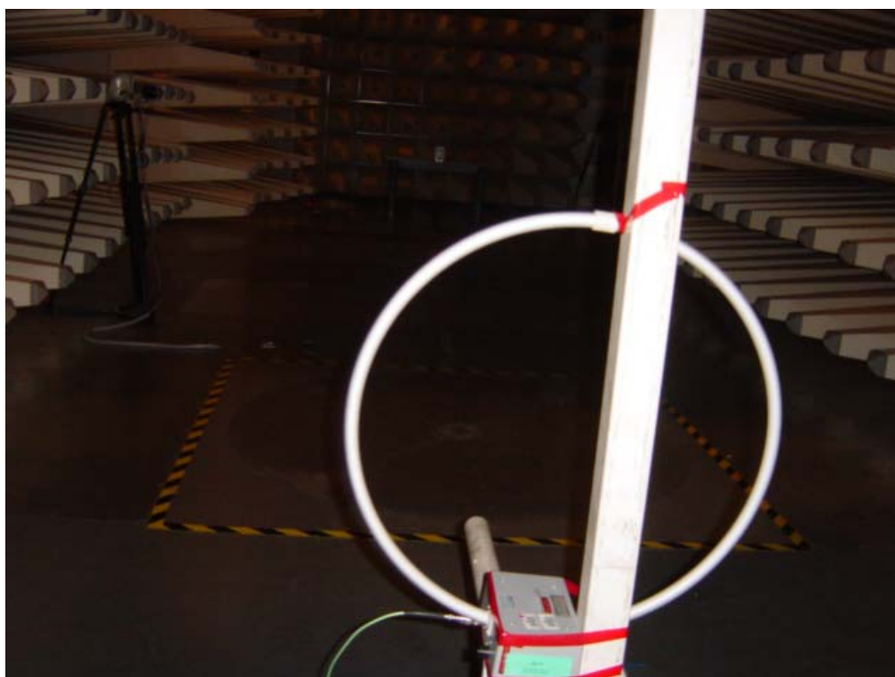
Set-up for Radiation Emission (Transmitter)
