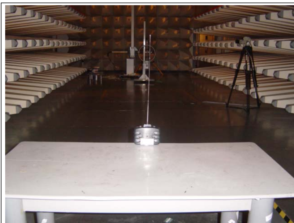
Set-up for Radiation Emission using Loop Antenna (Transmitter)
