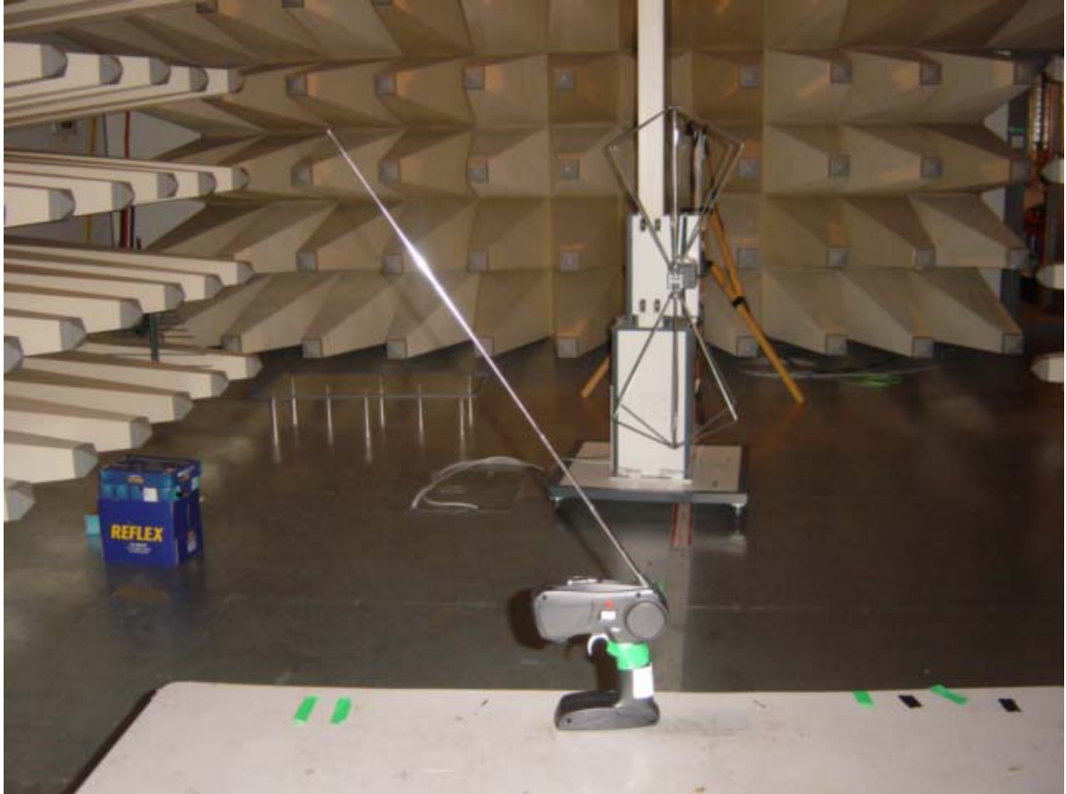
Set-up for Radiation Emission (Transmitter)
