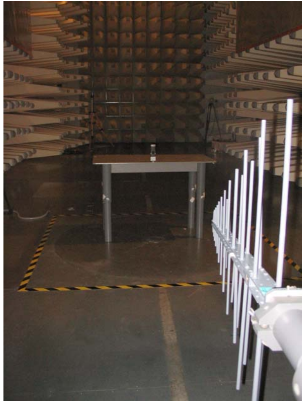
Set-up for Radiation Emission ( Transmitter)
