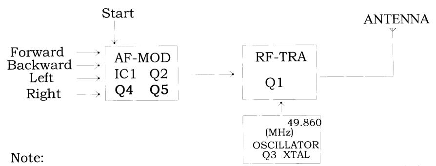
IC1, Q2,Q4,Q5 and the associated circuit act as AF-Modulator.
