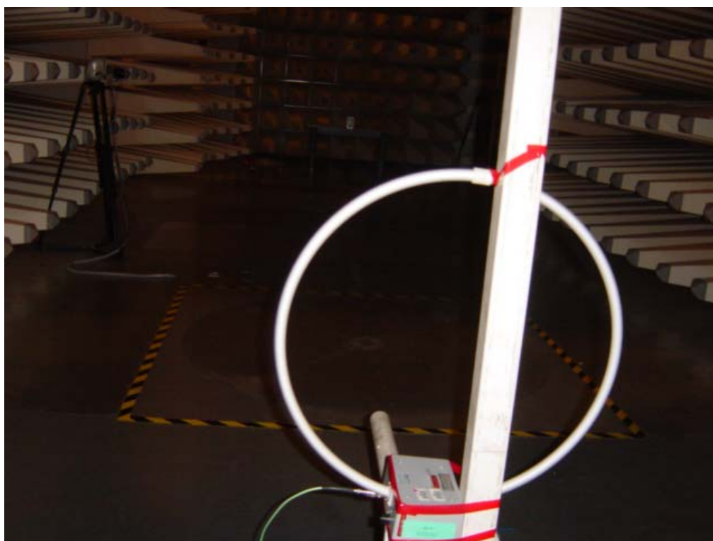
Set-up for Radiation Emission (Transmitter)
