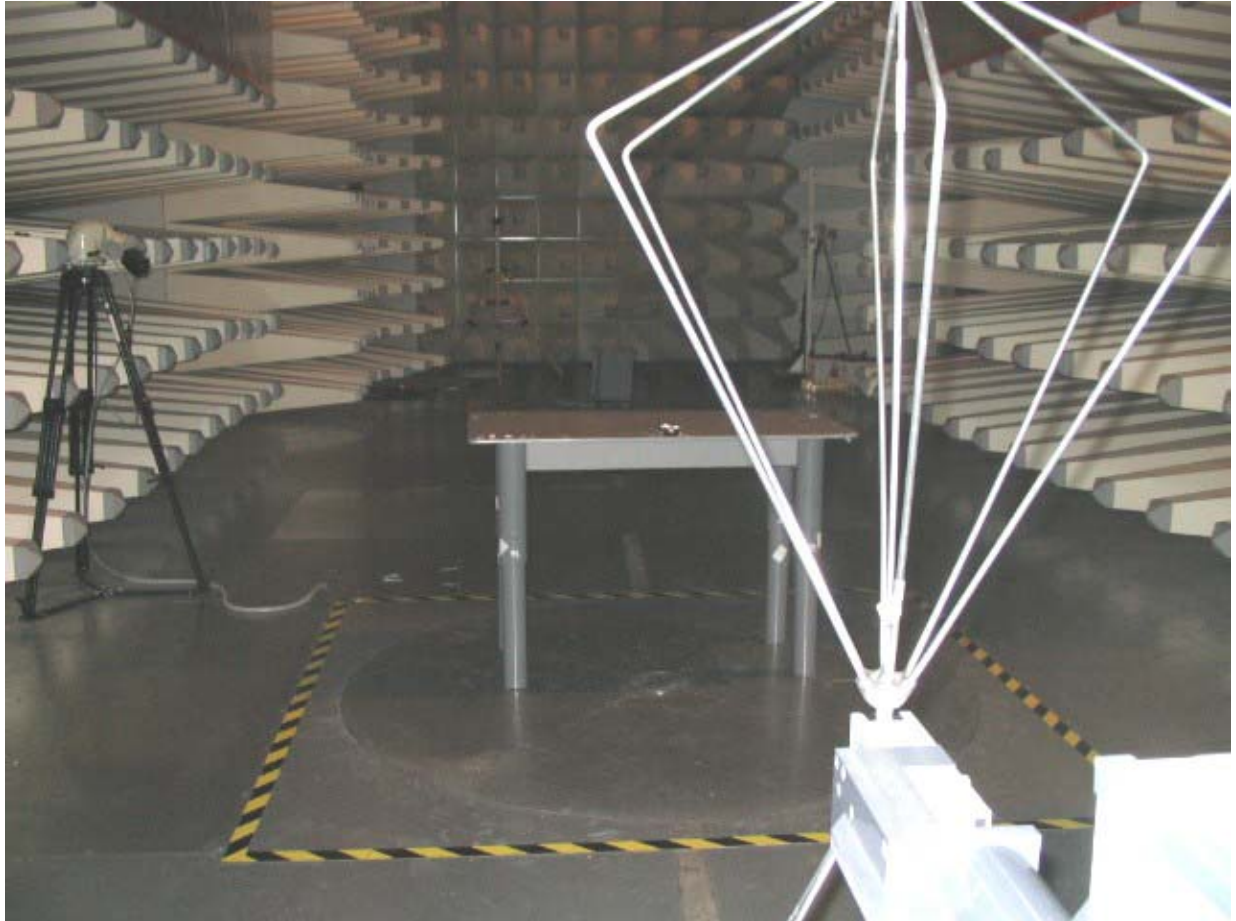
Set-up for Radiation Emission ( Receiver)
