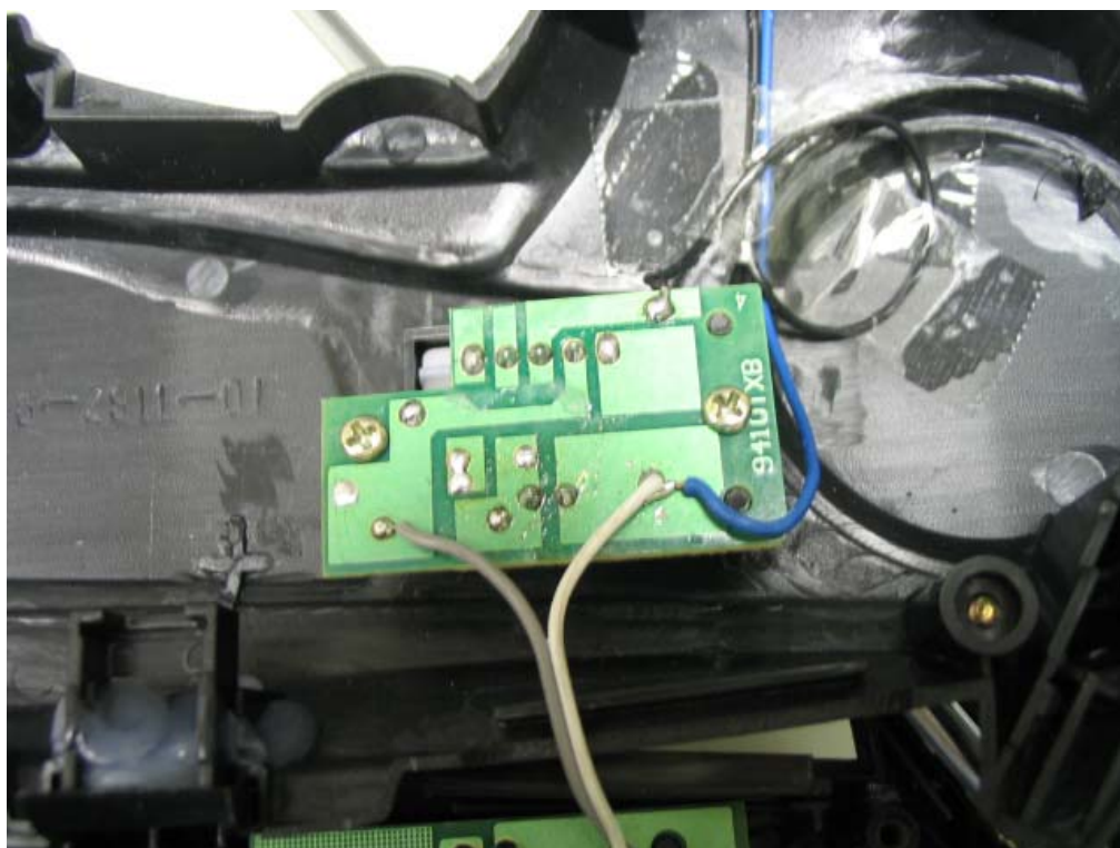
Transmitter (Internal view)
