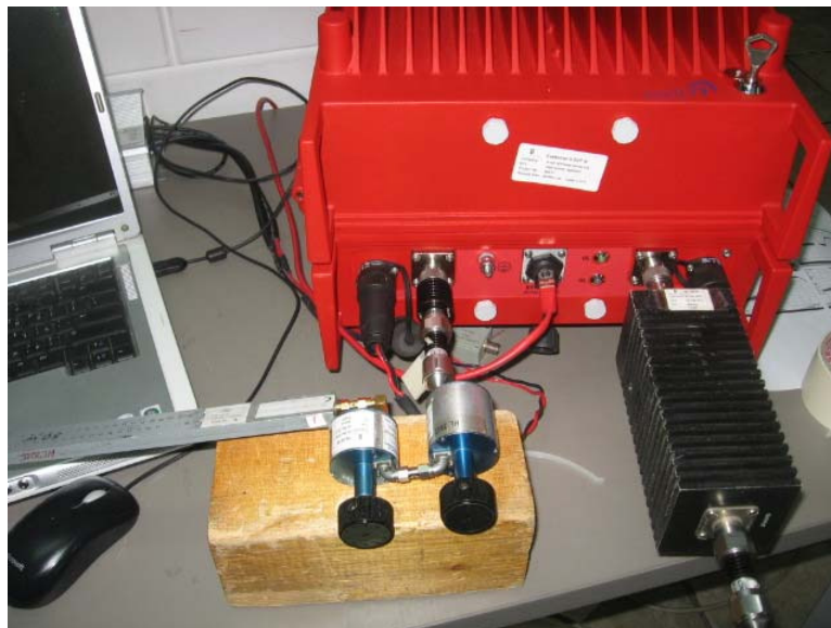
Photograph 7.8.1 Spurious emission test setup
