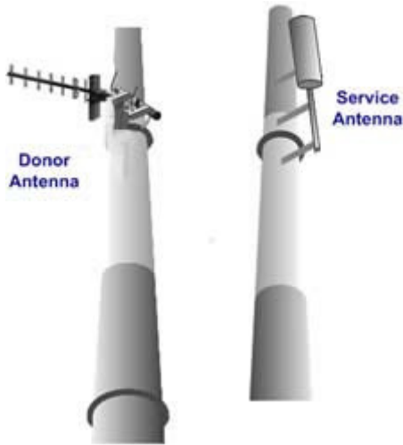
Figure 2-3. Donor and Service Antennas Installed on Separate Towers
