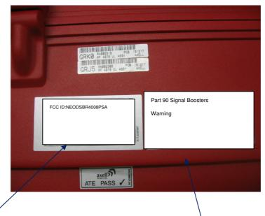
Label with FCC ID:NEODSBR4008PSA will be located here. The Warning label will be located here.
