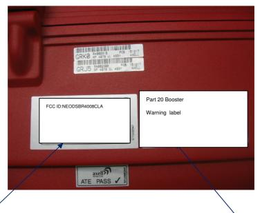
Label with FCC ID:NEODSBR4008CLA will be located here. The Warning label will be located here.
