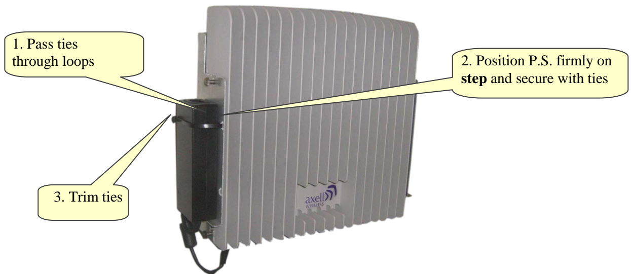
Figure 3-5. Mounting P.S.
