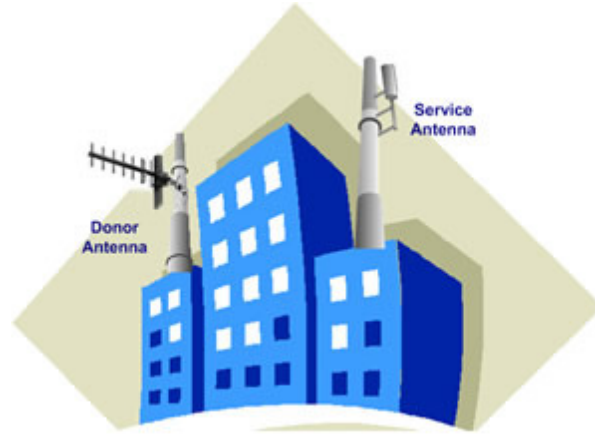
Figure 2-4. Service and Donor Antennas Installed on Opposite Sides of the Building
