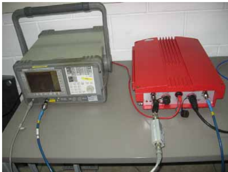
Photograph 7.8.1 Noise figure test setup
