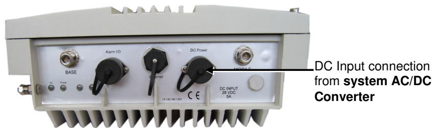
Figure 3-9. DC Power Input Connection Location
