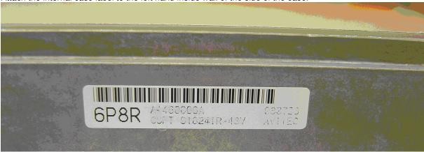
Attach the port designation label to the front edge of the case adjacent to the connector ports.
