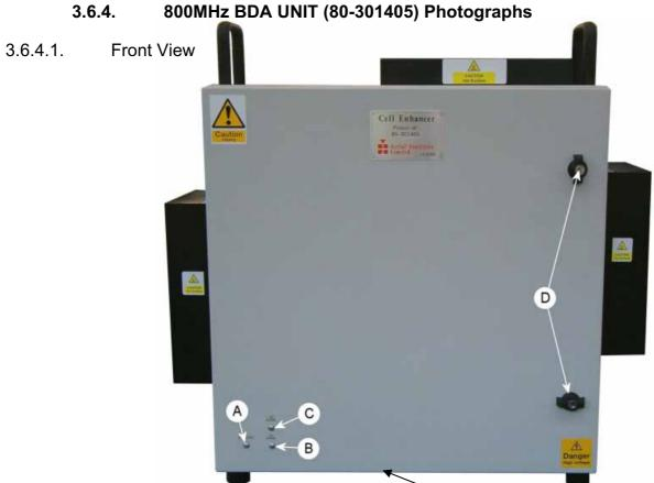
Note: All connectors (RF, DC and Alarms) are on the underside
