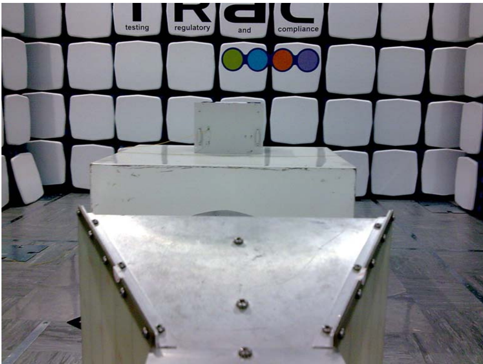
Photograph 2: Above 1 GHz Test Setup
