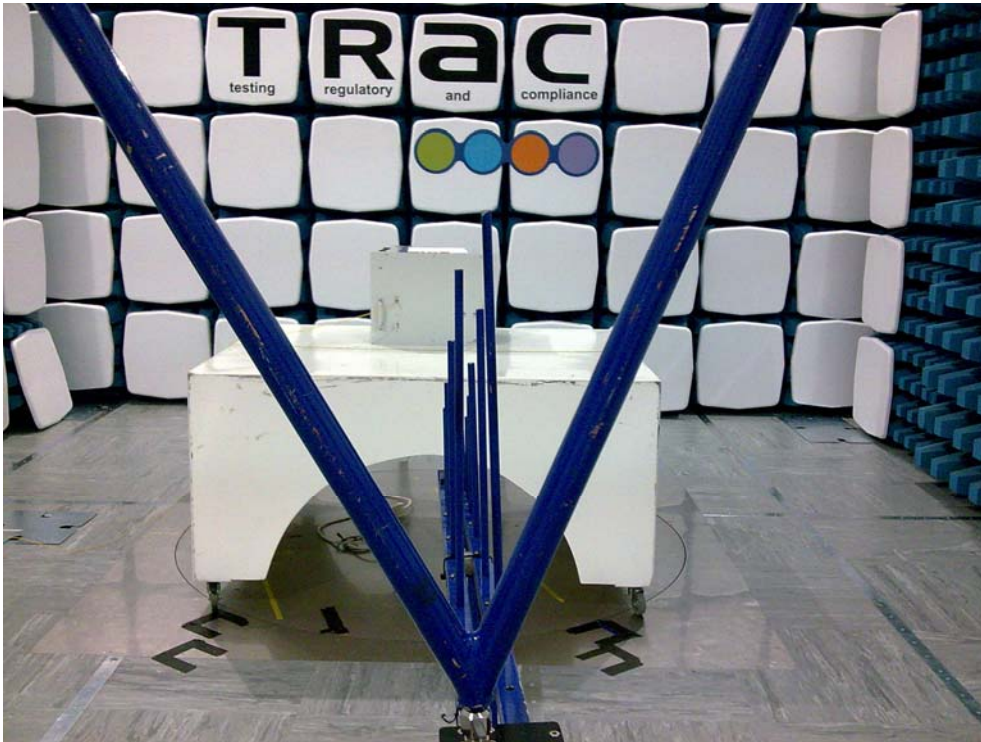
Photograph 1: 30 MHz to 1 GHz Test Setup
