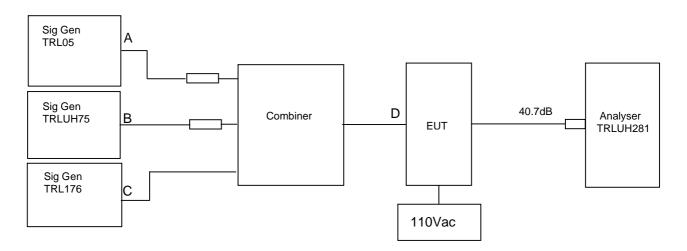
The intermodulation and spurious products were measured with the amplifier operating at maximum gain. A three tone test was conducted using the equipment as above. The input power level was adjusted so the level at point D was 10dB above the maximum input. The cable and attenuator loss between the EUT and the spectrum analyser was 30.3dB.
