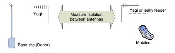
B). Install the equipment with gain set 10dB below the isolation figure obtained above
