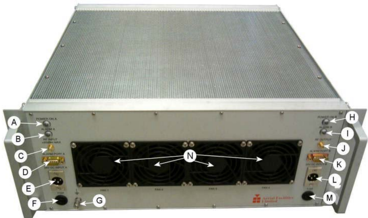
100W Linearised Amplifier (80-245101) front view
