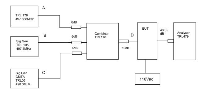
The intermodulation and spurious products were measured with the amplifier operating at maximum gain. A three tone test was conducted using the equipment as above. The input power level was adjusted so the level at point D was 10dB above the maximum input of –47.5.dBm. The cable and attenuator loss between the EUT and the spectrum analyser was 46.35dB.
