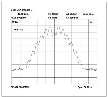
497.8 MHz Signal Generator and EUT, deviation set to 5kHz
