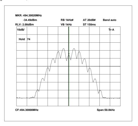
494.3 MHz Signal Generator and EUT, deviation set to 5kHz
