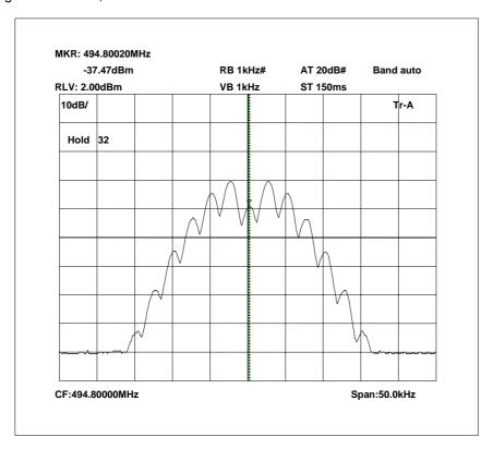
494.8 MHz Signal Generator and EUT, deviation set to 5kHz
