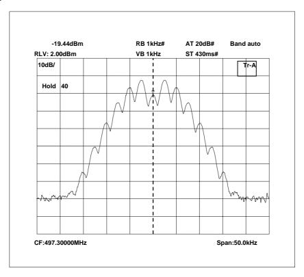
497.3 MHz Signal Generator and EUT, deviation set to 5kHz
