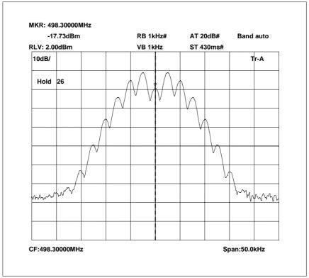
498.3 MHz Signal Generator and EUT, deviation set to 5kHz
