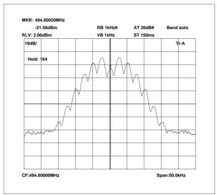
495.3 MHz Signal Generator, deviation set to 5kHz
