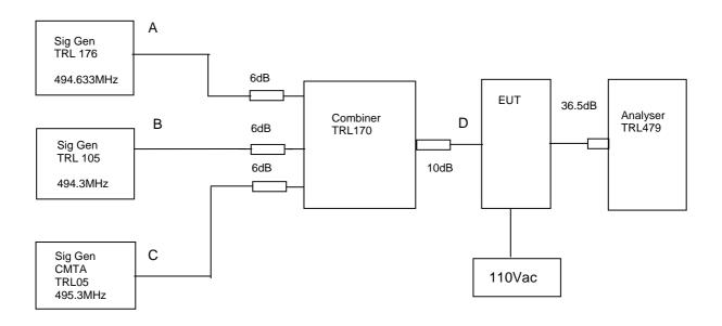
The Intermodulation and spurious products were measured with the amplifier operating at maximum gain. A three tone test was conducted using the equipment as above. The input power level was adjusted so the level at point D was 10 dB above the maximum input of -63dBm. The cable and attenuators loss between the EUT and the spectrum analyser was 36.5 dB.
