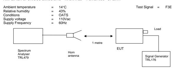
The test was set up as per the diagram. The level at the input was adjusted to compensate for the loss of the interconnecting cable. The unit was tested operating maximum power on three test frequencies with a 50 ohm load on the output. The unit was also tested with the signal generator replaced by another 50ohm load.
