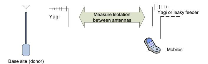
B). Install the Cell Enhancer with its gain set 10dB below the isolation figure obtained above.
