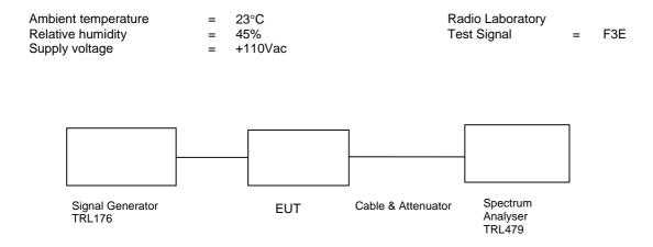
The test was set up as per the diagram. The level at the input was adjusted to compensate for the loss of the interconnecting cable. The unit was tested operating at maximum power and on three test frequencies.
