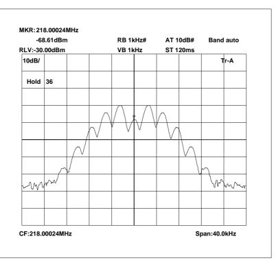
218.0 MHz Signal Generator and EUT, deviation set to 5kHz
