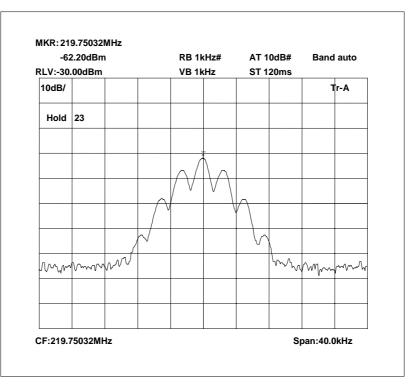
219.75 MHz Signal Generator, deviation set to 5kHz
