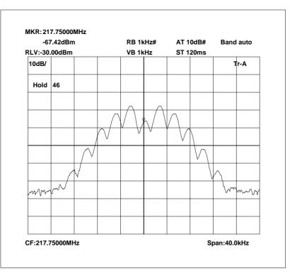
217.75 MHz Signal Generator, deviation set to 5kHz
