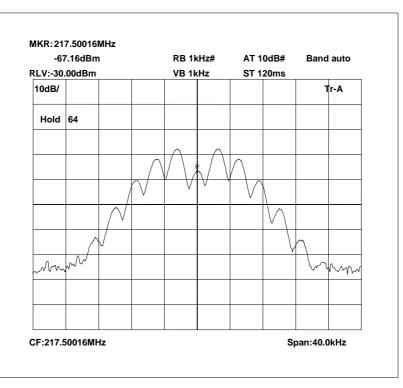
217.5 MHz Signal Generator and EUT, deviation set to 5kHz
