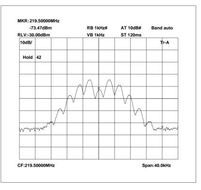
219.5 MHz Signal Generator and EUT, deviation set to 5kHz
