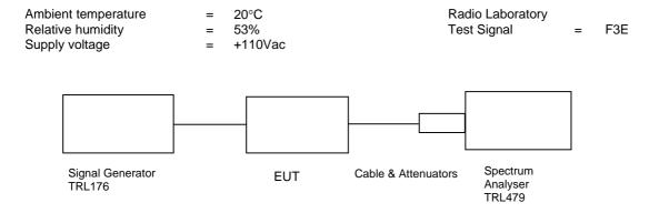
The test was set up as per the diagram. The level at the input was adjusted to compensate for the loss of the interconnecting cable. The unit was tested operating at maximum power and on three test frequencies.
