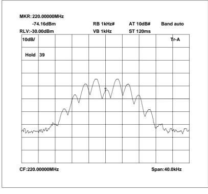
220.0 MHz Signal Generator, deviation set to 5kHz
