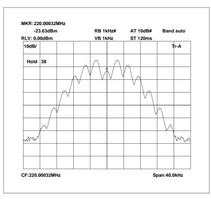
The above plots depicting the output waveshape show no measurable distortion visible when compared to the input signal.
