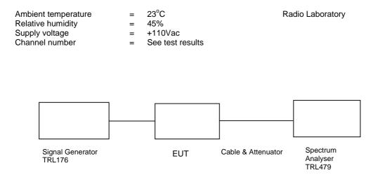
This test was performed to show that the amplifier does not alter the input signal in any way. The input signal was set to the maximum input level (-60.0dBm) and modulated with a 2500Hz tone. The plots show the signal measured at the signal generator and the signal measured at the output of the EUT.
