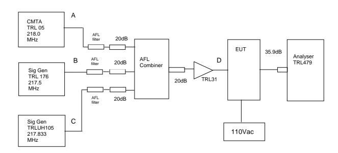
The Intermodulation and spurious products were measured with the amplifier operating at maximum gain. A three tone test was conducted using the equipment as above. The input power level was adjusted so the level at point D was 10dB above the maximum input of -7dBm.The cable and attenuators loss between the EUT and the spectrum analyser was 35.9 dB.
