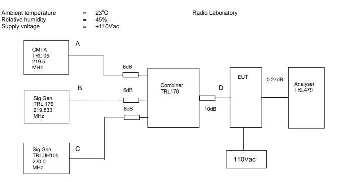
The Intermodulation and spurious products were measured with the amplifier operating at maximum gain. A three tone test was conducted using the equipment as above. The input power level was adjusted so the level at point D was 10db above the maximum input of -60.0dBm.The cable and attenuator loss between the EUT and the spectrum analyser was 0.27dB.
