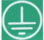
Cell Enhancers supplied from the mains must be connected to grounded outlets and earthed in conformity with appropriate local, national and international electricity supply and safety regulations.
