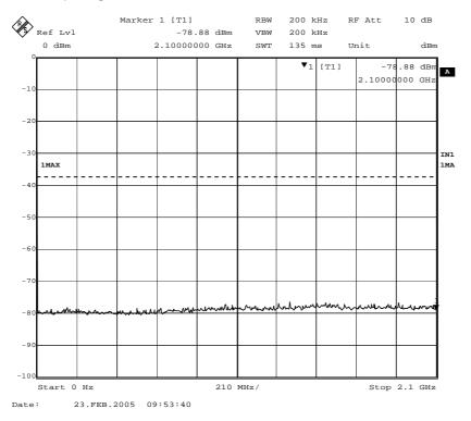
Radiated emissions no input signal 2.1 - 4.2GHz
