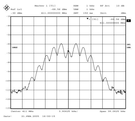
411.0 MHz Signal Generator and EUT, deviation set to 5kHz
