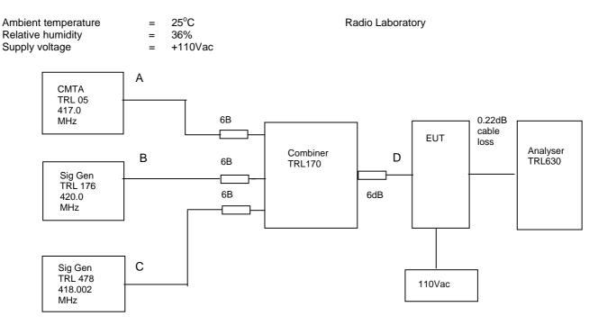
The Intermodulation and spurious products were measured with the amplifier operating at maximum gain. A three tone test was conducted using the equipment as above. The input power level was adjusted so the level at point D was 10dB above the maximum input of -51dm.The cable loss between the EUT and the spectrum analyser was 0.22
