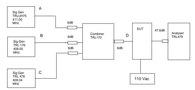
The Intermodulation and spurious products were measured with the amplifier operating at maximum gain. A three tone test was conducted using the equipment as above. The input power level was adjusted so that the level at point D was 10dB above the maximum input of -12.5dBm.The cable and attenuators loss between the EUT and the spectrum analyser was 47.6dB.
