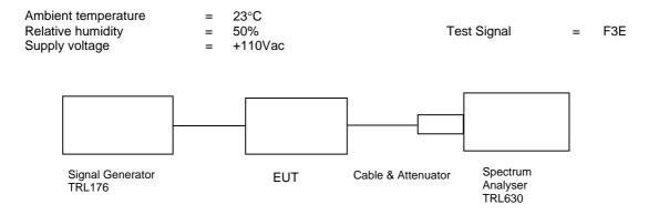
The test was set up as per the diagram. The level at the input was adjusted to compensate for the loss of the interconnecting cable. The unit was tested operating at maximum power and on three test frequencies.
