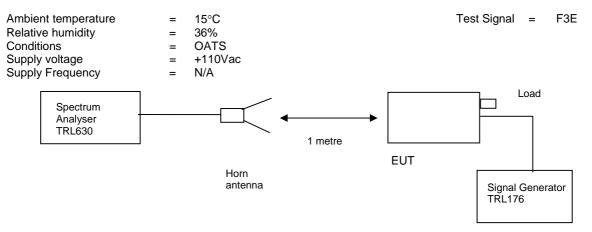
The test was set up as per the diagram. The level at the input was adjusted to compensate for the loss of the interconnecting cable. The unit was tested operating maximum power on three test frequencies with a 50 ohm load on the output. The unit was also tested with the signal generator replaced by another 50 ohm load.
