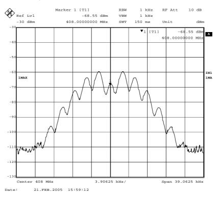
408.0 MHz Signal Generator and EUT, deviation set to 5kHz
