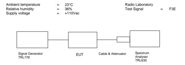
The test was set up as per the diagram. The level at the input was adjusted to compensate for the loss of the interconnecting cable. The unit was tested operating at maximum power and on three test frequencies.
