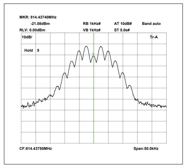
814.4375MHz Signal Generator and amplifier deviation set to 5kHz
