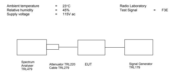
The test was set up as per the diagram. The level at the input was adjusted to compensate for the loss of the interconnecting cable. The unit was tested operating at maximum power and on three test frequencies.
