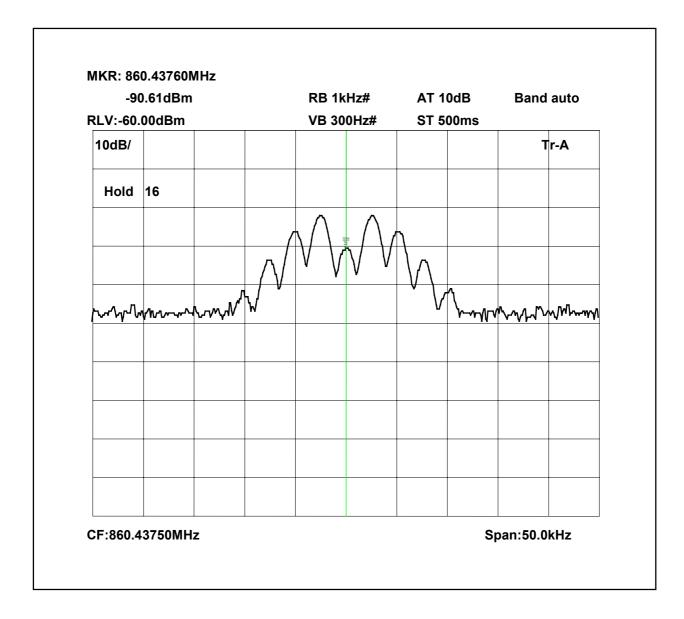
860.4375MHz Signal Generator deviation set to 5kHz
