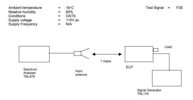
The test was set up as per the diagram. The level at the input was adjusted to compensate for the loss of the interconnecting cable. The unit was tested operating maximum power on three test frequencies with a 50 ohm load on the output. The unit was also tested with the signal generator replaced by another 50 ohm load.
