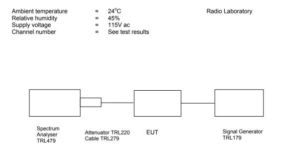
This test was performed to show that the amplifier does not alter the input signal in any way. The input signal was set to the maximum input level (-73.1dBm) and modulated with a 2500Hz tone. The plots show the signal measured at the signal generator and the signal measured at the output of the EUT.
