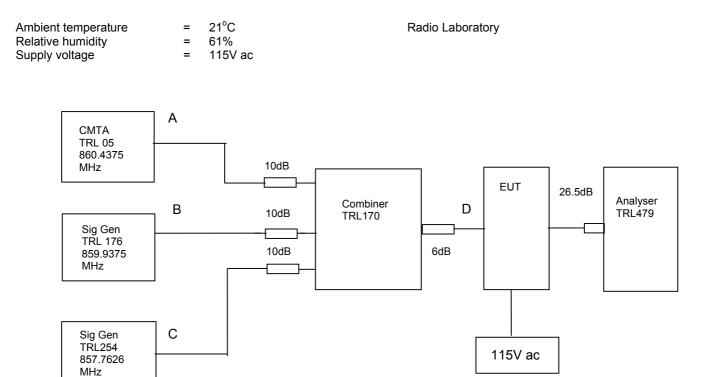
The Intermodualation and spurious products were measured with the amplifier operating at maximum gain. A three tone test was conducted using the equipment as above. The input power level was adjusted so the level at point D was the maximum input of –77.4dBm. The cable and attenuator loss between the EUT and the spectrum analyser was 26.57dB.
