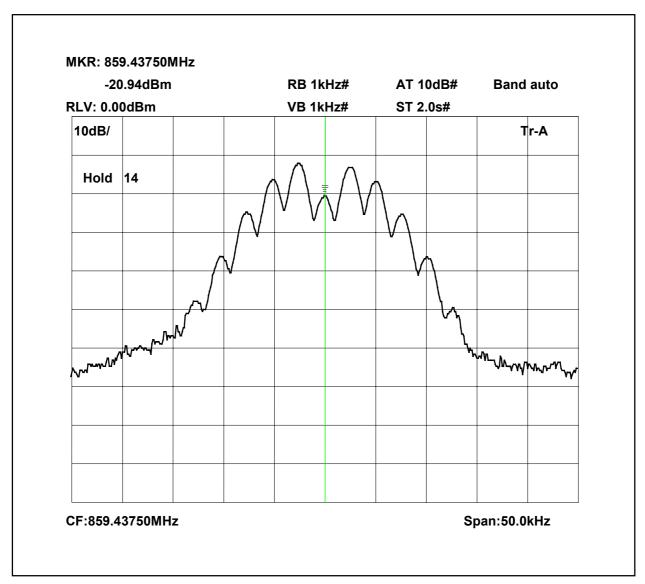
859.4375MHz Signal Generator and amplifier deviation set to 5kHz
