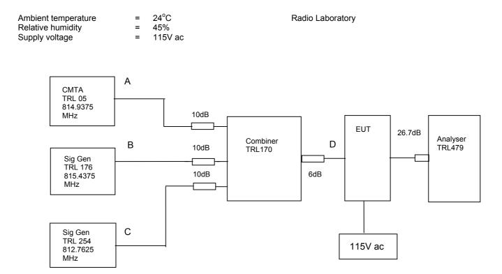
The Intermodualation and spurious products were measured with the amplifier operating at maximum gain. A three tone test was conducted using the equipment as above. The input power level was adjusted so the level at point D was the maximum input of –77.3dBm The cable and attenuator loss between the EUT and the spectrum analyser was 26.62dB.
