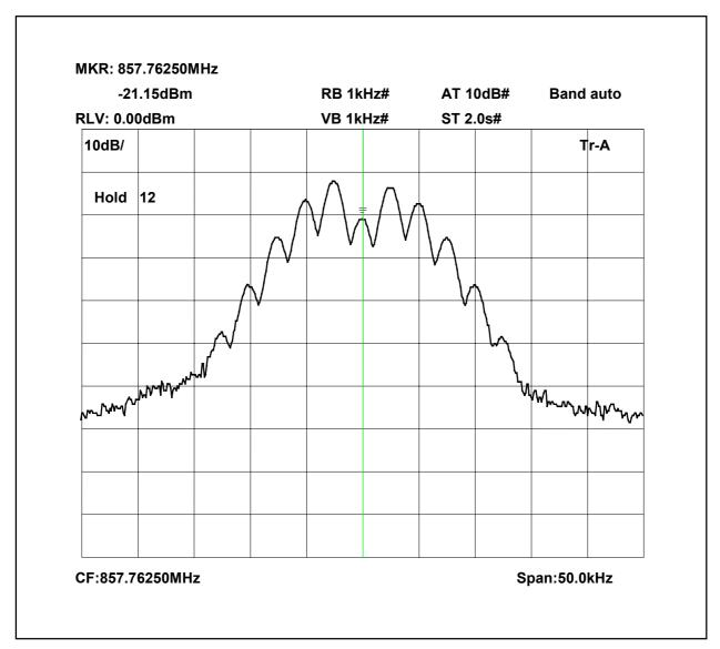
857.7625MHz Signal Generator and EUT deviation set to 5kHz
