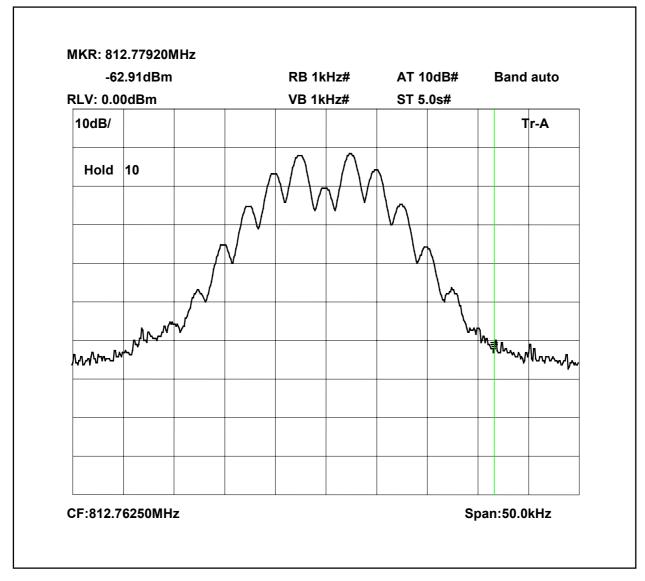
812.7625MHz Signal Generator and EUT deviation set to 5kHz
