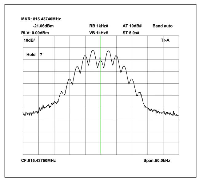
815.4375MHz Signal Generator deviation set to 5kHz
