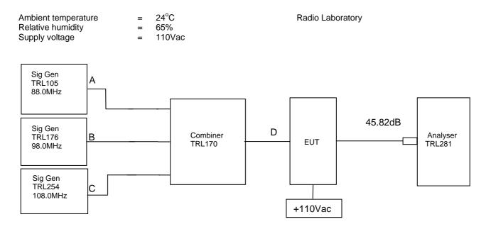
The intermodulation and spurious products were measured with the amplifier operating at maximum gain. A three tone test was conducted using the equipment as above. The signal input power level was adjusted until the amplifier reached the +1dB compression point across the three carriers, the signal input power level was then increased by 10dB (-17dBm). The cable and attenuator loss between the EUT and the spectrum analyser was 45.82dB.
