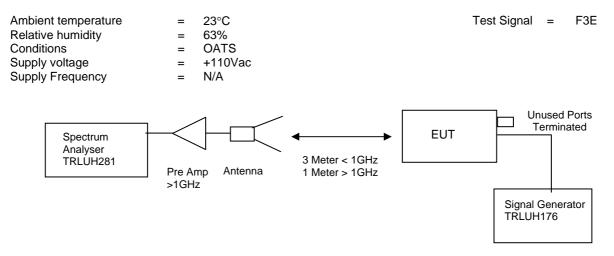
The test was set up as per the diagram. The level at the input was adjusted to compensate for the loss of the interconnecting cable. The unit was tested operating maximum power on three test frequencies with a 50 ohm load on the output.
