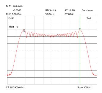
The above plots depicting the out waveshape show no measurable distortion visible when compared to the input signal.
