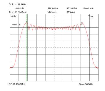
Bottom channel 87.9MHz Signal Generator and EUT, deviation set to 100.0kHz
