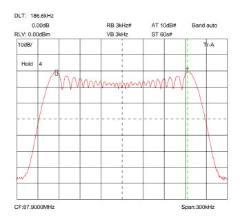
Middle channel 98.0MHz Signal Generator, deviation set to 100.0kHz
