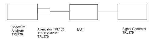
This test was performed to show that the amplifier does not alter the input signal in any way. The input signal was set to the maximum input level (-55.4Bm) and modulated with a 2500Hz tone. The plots show the signal measured at the signal generator and the signal measured at the output of the EUT.
