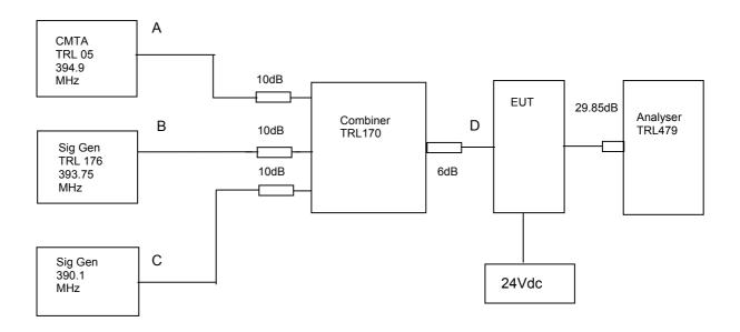
The Intermodulation and spurious products were measured with the amplifier operating at maximum gain. A three tone test was conducted using the equipment as above. The input power level was adjusted so the level at point D was the maximum input of -53.4dBm The cable and attenuators loss between the EUT and the spectrum analyser was 29.85 dB.
