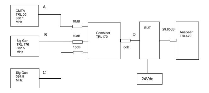
The Intermodulation and spurious products were measured with the amplifier operating at maximum gain. A three tone test was conducted using the equipment as above. The input power level was adjusted so the level at point D was the maximum input of –61.4dBm. The cable and attenuator loss between the EUT and the spectrum analyser was 29.85dB.
