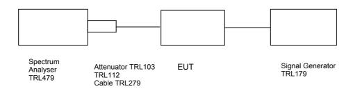
The test was set up as per the diagram. The level at the input was adjusted to compensate for the loss of the interconnecting cable. The unit was tested operating at maximum power and on three test frequencies.
