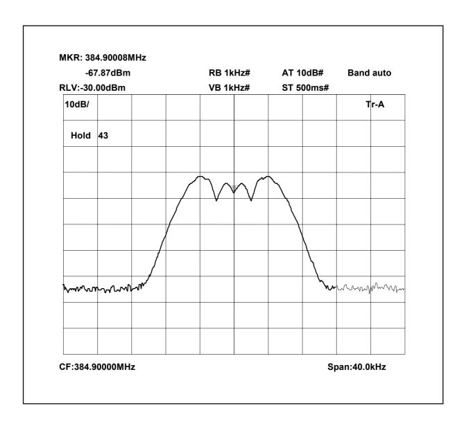
384.9MHz Signal Generator deviation set to 5kHz
