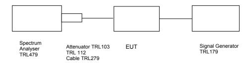
This test was performed to show that the amplifier does not alter the input signal in any way. The input signal was set to the maximum input level (-61.4 dBm) and modulated with a 2500Hz tone. The plots show the signal measured at the signal generator and the signal measured at the output of the EUT.
