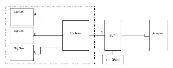
Signal Generator B was varied in frequency to check if intermodulation products where produced.
