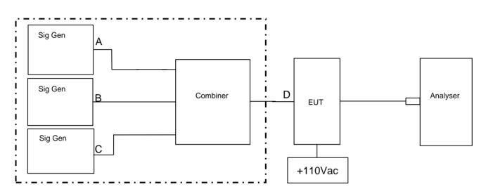
Signal Generator B was varied in frequency to check if intermodulation products where produced.
