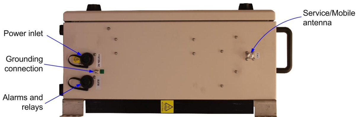
Figure 1-2. D-CSR Door Locks and Left Side Panel Interfaces
