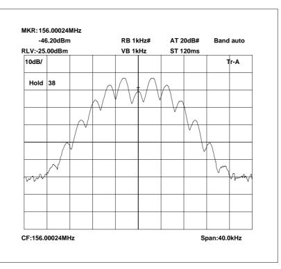
156.0 MHz Signal Generator and EUT, deviation set to 5kHz
