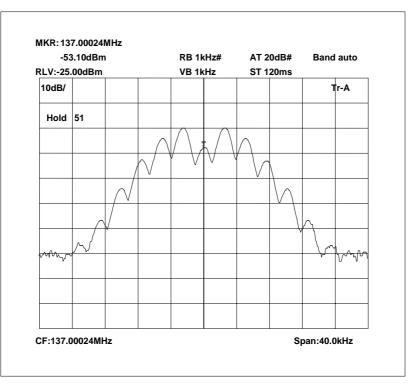
137.0 MHz Signal Generator and EUT, deviation set to 5kHz
