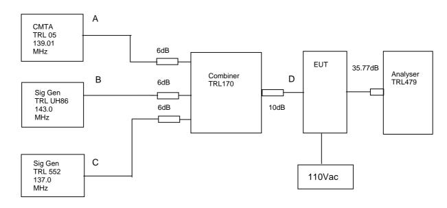
The Intermodulation and spurious products were measured with the amplifier operating at maximum gain. A three tone test was conducted using the equipment as above. The input power level was adjusted so the level at point D was 10 dB above the maximum input of -4.5dBm.The cable and attenuator loss between the EUT and the spectrum analyser was 35.77dB.
