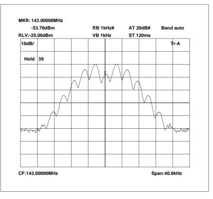
143.0 MHz Signal Generator and EUT, deviation set to 5kHz
