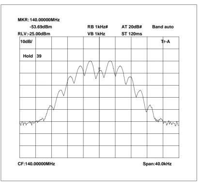
140.0 MHz Signal Generator, deviation set to 5kHz
