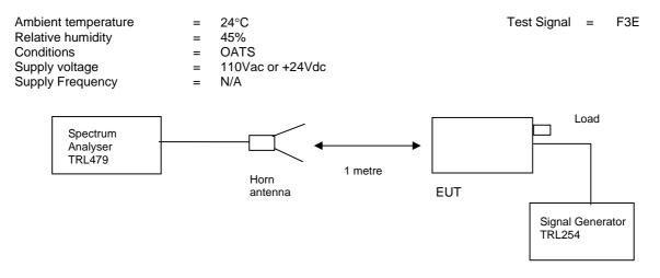
The test was set up as per the diagram. The level at the input was adjusted to compensate for the loss of the interconnecting cable. The unit was tested operating maximum power on three test frequencies with a 50 ohm load on the output. The unit was also tested with the signal generator replaced by another 50 ohm load.
