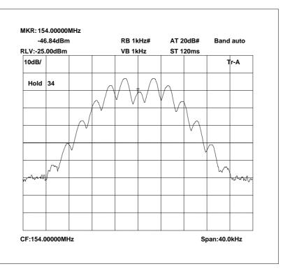
154.0 MHz Signal Generator and EUT, deviation set to 5kHz
