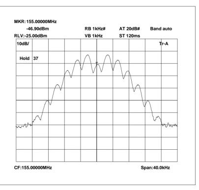
155.0 MHz Signal Generator and EUT, deviation set to 5kHz
