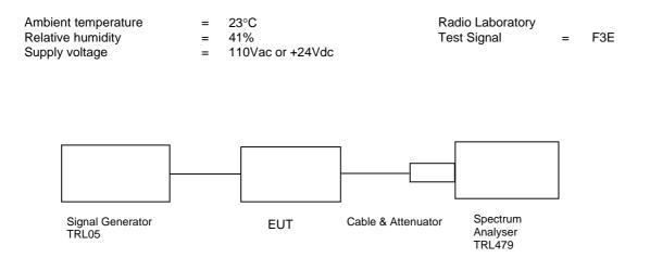
The test was set up as per the diagram. The level at the input was adjusted to compensate for the loss of the interconnecting cable. The unit was tested operating at maximum power and on three test frequencies.
