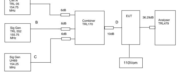
The Intermodulation and spurious products were measured with the amplifier operating at maximum gain. A three tone test was conducted using the equipment as above. The input power level was adjusted so the level at point D was 10dB above the maximum input of +3dBm. The cable and attenuators loss between the EUT and the spectrum analyser was 36.29 dB.
