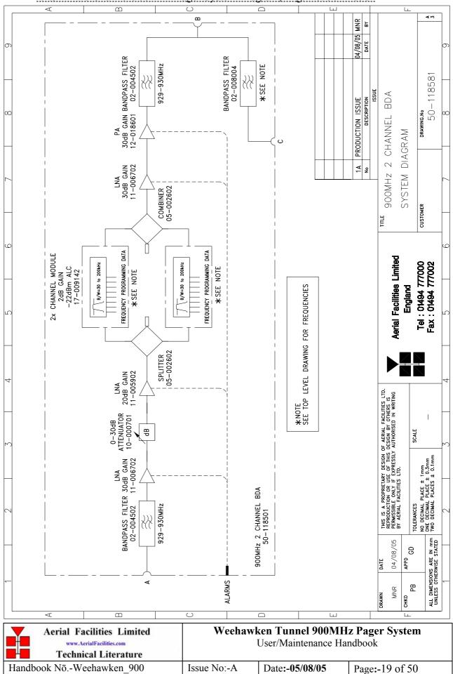
4.1.3 Two Channel 900MHz Pager System Diagram, Drg. No. 50-118581
