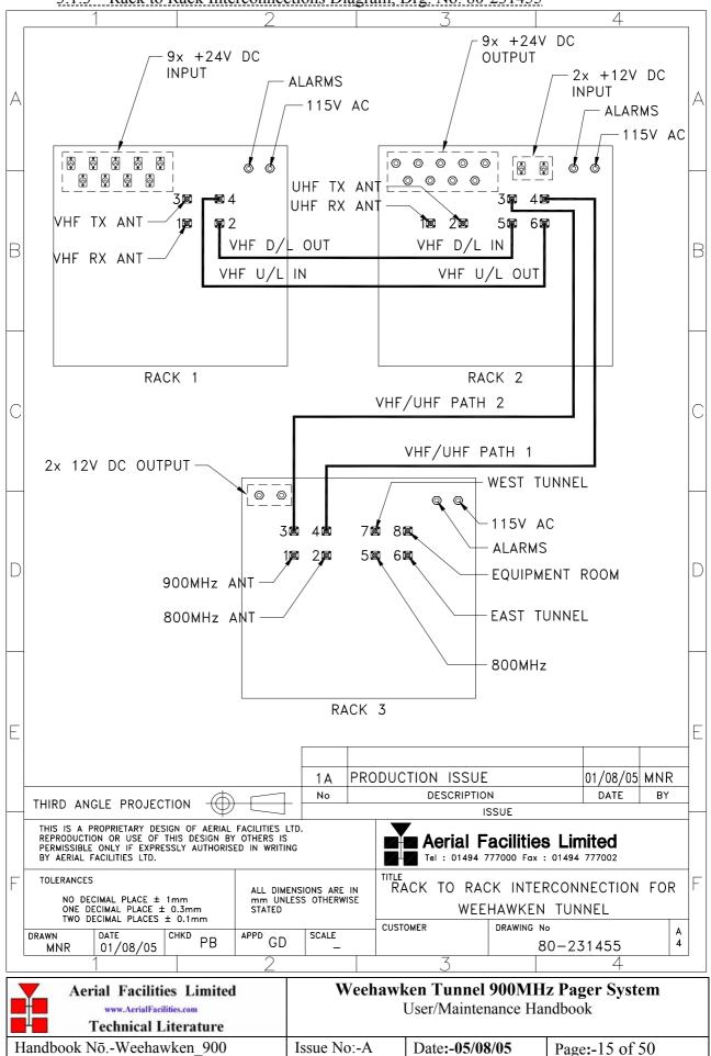
3.1.3 Rack to Rack Interconnections Diagram, Drg. No. 80-231455
