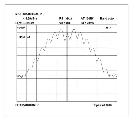
824.0 MHz Signal Generator deviation set to 5kHz
