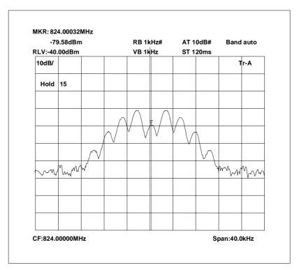
824.0 MHz Signal Generator and EUT deviation set to 5kHz
