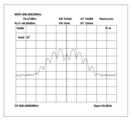
806.0 MHz Signal Generator and EUT deviation set to 5kHz
