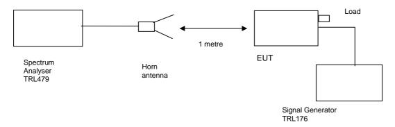
The test was set up as per the diagram. The level at the input was adjusted to compensate for the loss of the interconnecting cable. The unit was tested operating maximum power on three test frequencies with a 50 ohm load on the output.
