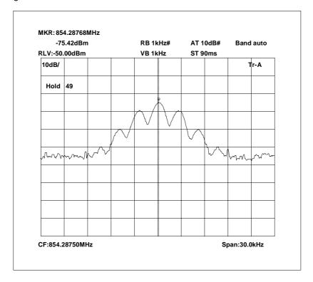
854.2875 MHz Signal Generator and EUT deviation set to 2.5kHz
