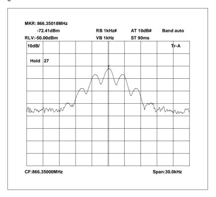
866.3500 MHz Signal Generator and EUT deviation set to 2.5kHz
