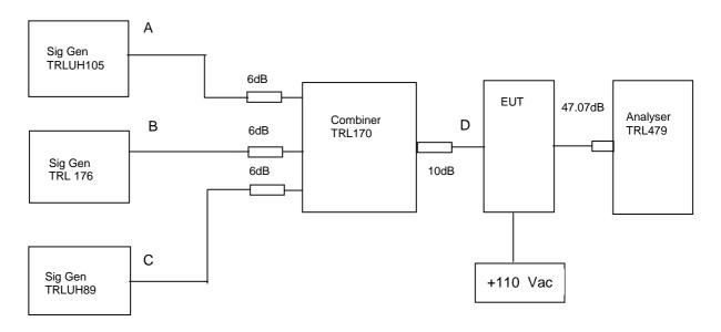
The Intermodulation and spurious products were measured with the amplifier operating at maximum gain. A three tone test was conducted using the equipment as above. The input power level was adjusted so the level at point D was the maximum input of -65dBm. The cable and attenuator loss between the EUT and the spectrum analyser was 47.07dB. This test was performed on the frequencies listed in the table below. Sweep data is shown on the next page for scan with the highest intermodulation product:
