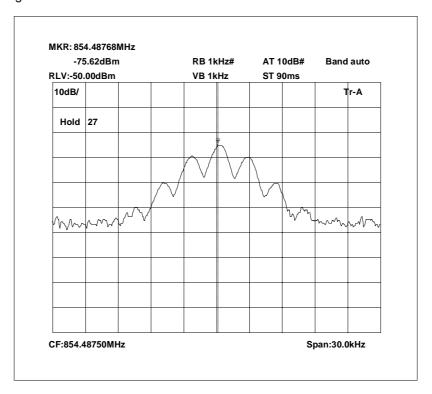
854.4875 MHz Signal Generator and EUT deviation set to 2.5kHz
