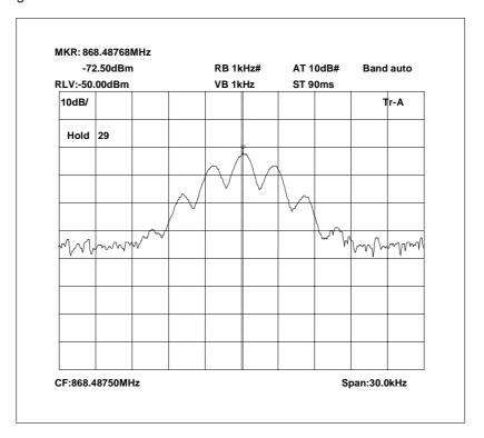
868.4875 MHz Signal Generator and EUT deviation set to 2.5kHz
