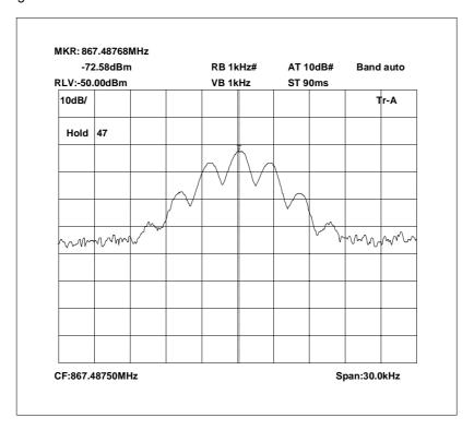
867.4875 MHz Signal Generator and EUT deviation set to 2.5kHz
