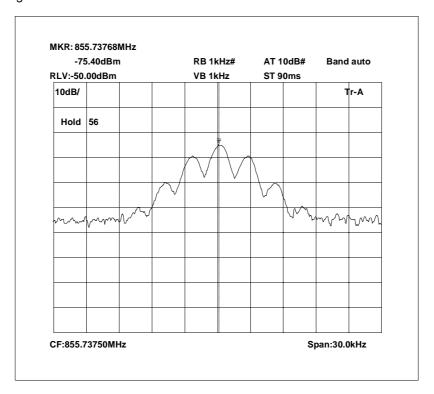
855.7375 MHz Signal Generator and EUT deviation set to 2.5kHz
