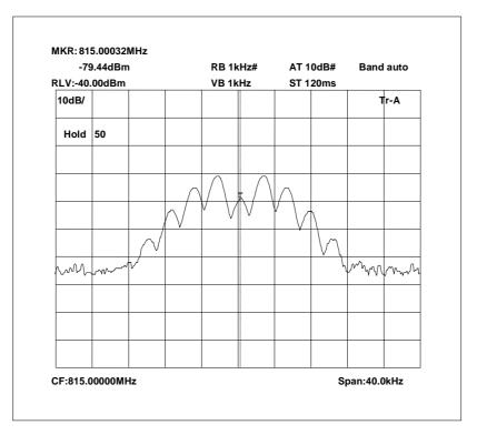
815.0 MHz Signal Generator and EUT deviation set to 5kHz
