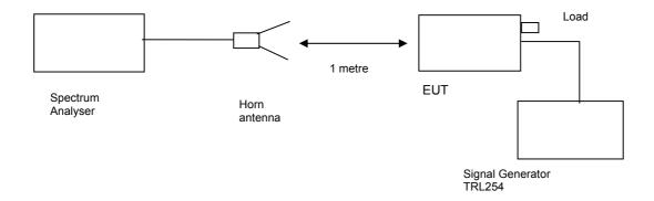
The test was set up as per the diagram. The level at the input was adjusted to compensate for the loss of the interconnecting cable. The unit was tested operating maximum power on three test frequencies with a 50 ohm load connected to the output. The unit was also tested with the signal generator replaced by another 50ohm load.
