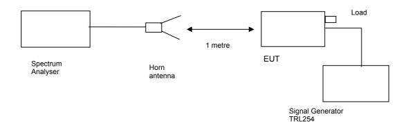
The test was set up as per the diagram. The level at the input was adjusted to compensate for the loss of the interconnecting cable. The unit was tested operating maximum power on three test frequencies with a 50 ohm load connected to the output. The unit was also tested with the signal generator replaced by another 50ohm load. The EUT's downlink path had 10dB's of internal attenuation switched in.
