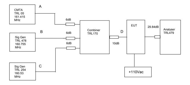
The Intermodulation and spurious products were measured with the amplifier operating at maximum gain. A three tone test was conducted using the equipment as above. The input power level was adjusted so the level at point D was the maximum input of -82.2dBm. The cable and attenuator loss between the EUT and the spectrum analyser was 29.84dB. This loss was taken into account by adjusting the analysers level offset.
