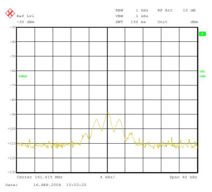
161.415 Signal Generator deviation set to 2.5kHz
