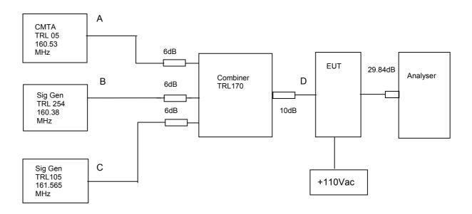
The Intermodulation and spurious products were measured with the amplifier operating at maximum gain. A three tone test was conducted using the equipment as above. The input power level was adjusted so the level at point D was the maximum input of -78.83dBm. The cable and attenuators loss between the EUT and the spectrum analyser was 29.84 dB. The EUT's downlink path had 10dB's of internal attenuation switched in.
