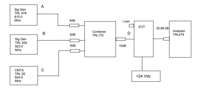
The intermodulation and spurious products were measured with the amplifier operating at maximum gain. A three tone test was conducted using the equipment as above. The input power level was adjusted so the level at point D was the maximum input of -8.03dBm. The cable and attenuator loss between the EUT and the spectrum analyser was 30.68dB. This loss was taken into account by adjusting the analysers level offset.
