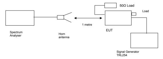
The test was set up as per the diagram. The level at the input was adjusted to compensate for the loss of the interconnecting cable. The unit was tested operating maximum power on three test frequencies with a 50 ohm load on the output. The unit was also tested with the signal generator replaced by another 50ohm load.
