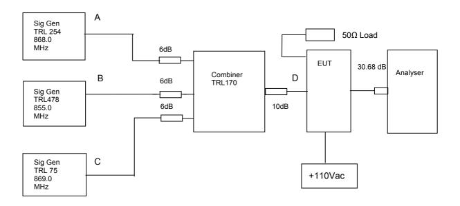
The intermodulation and spurious products were measured with the amplifier operating at maximum gain. A three tone test was conducted using the equipment as above. The input power level was adjusted so the level at point D was the maximum input of -7.63dBm. The cable and attenuators loss between the EUT and the spectrum analyser was 30.68 dB.
