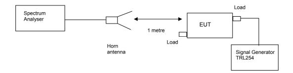
The test was set up as per the diagram. The level at the input was adjusted to compensate for the loss of the interconnecting cable. The unit was tested operating maximum power on three test frequencies with a 50 ohm load on the output. The unit was also tested with the signal generator replaced by another 50ohm load.
