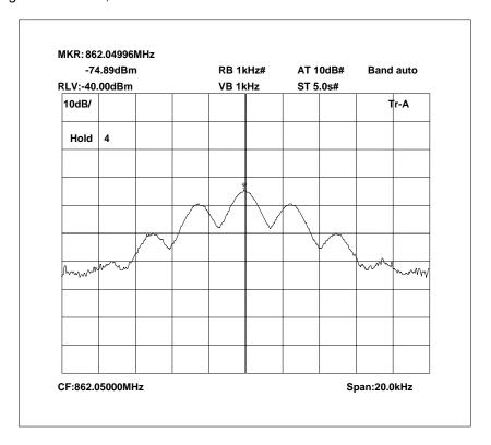
862.050 MHz Signal Generator and EUT, deviation set to 2.5kHz
