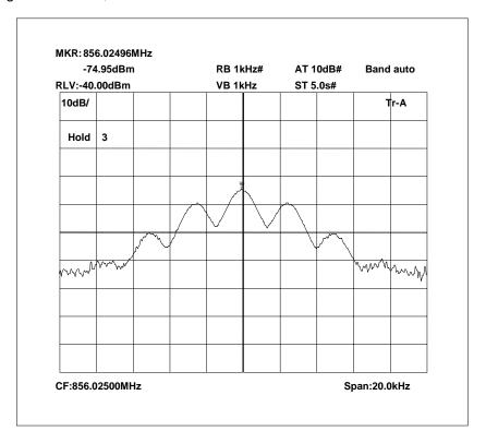
856.025 MHz Signal Generator and EUT, deviation set to 2.5kHz
