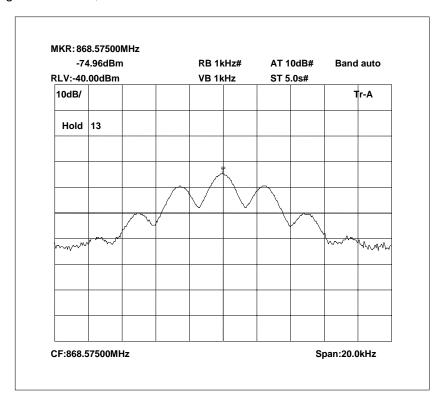
868.575 MHz Signal Generator and EUT, deviation set to 2.5kHz
