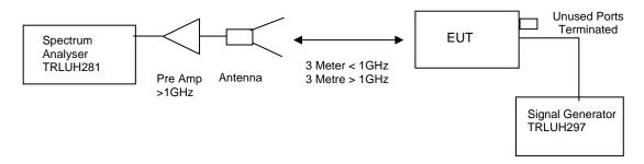
The test was set up as per the diagram. The level at the input was adjusted to compensate for the loss of the interconnecting cable. The unit was tested operating maximum power on three test frequencies with a 50 ohm load on the output. The unit was also tested with the signal generator replaced by another 50ohm load.
