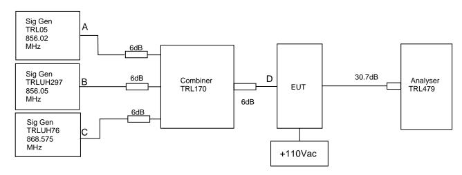
The intermodulation and spurious products were measured with the amplifier operating at maximum gain. A three tone test was conducted using the equipment as above. The input power level was adjusted so the level at point D was 10dB above the maximum input of -72dBm. The cable and attenuator loss between the EUT and the spectrum analyser was 30.7dB.
