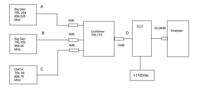
The intermodulation and spurious products were measured with the amplifier operating at maximum gain. A three tone test was conducted using the equipment as above. The input power level was adjusted so the level at point D was the maximum input of –63.4dBm. The cable and attenuators loss between the EUT and the spectrum analyser was 29.84 dB.
