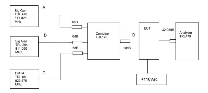
The intermodulation and spurious products were measured with the amplifier operating at maximum gain. A three tone test was conducted using the equipment as above. The input power level was adjusted so the level at point D was the maximum input of -74dBm. The cable and attenuator loss between the EUT and the spectrum analyser was 32.08dB. This loss was taken into account by adjusting the analysers level offset.
