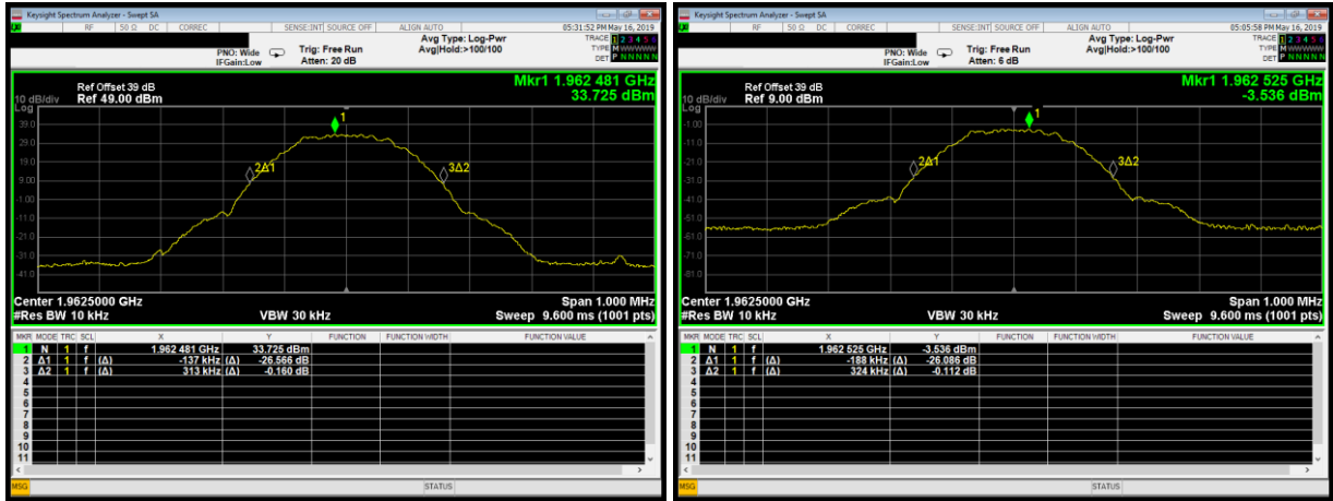
Plot 3.2.1: Input-versus-output signal comparison, MSK, Gaussian filter 0.3, data rate 270kbps, 0.5 dB below AGC threshold level
