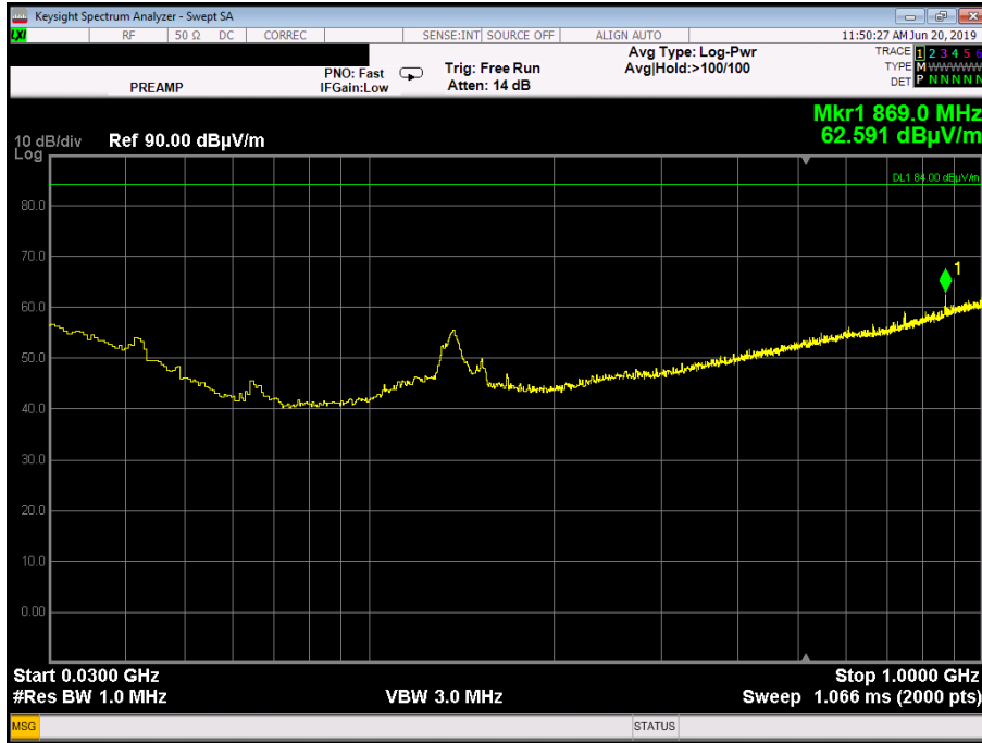
Plot 3.6.9: Spurious Emissions test results, 30 MHz – 1GHz range, Horizontal polarization, High Frequency
