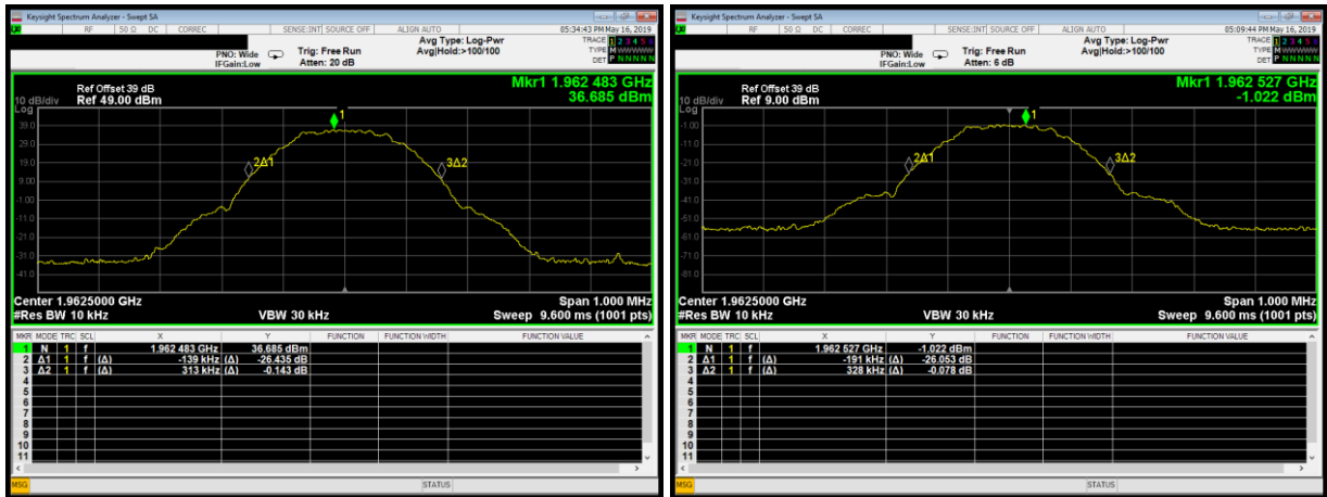
Plot 3.2.2: Input-versus-output signal comparison, MSK, Gaussian filter 0.3, data rate 270kbps, 3 dB above AGC threshold level
