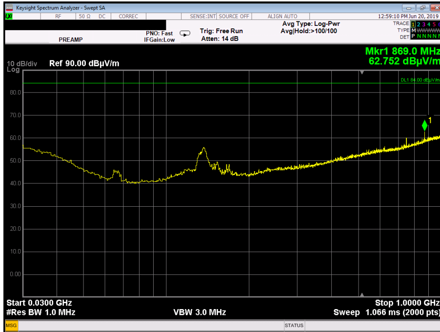
Plot 3.6.2: Spurious Emissions test results, 30 MHz – 1 GHz range, Vertical polarization, Low Frequency
